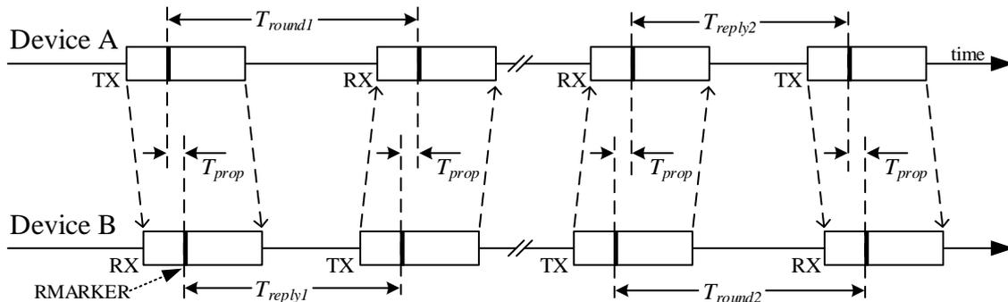
**Figure 37: Double-sided two-way ranging with four messages**
