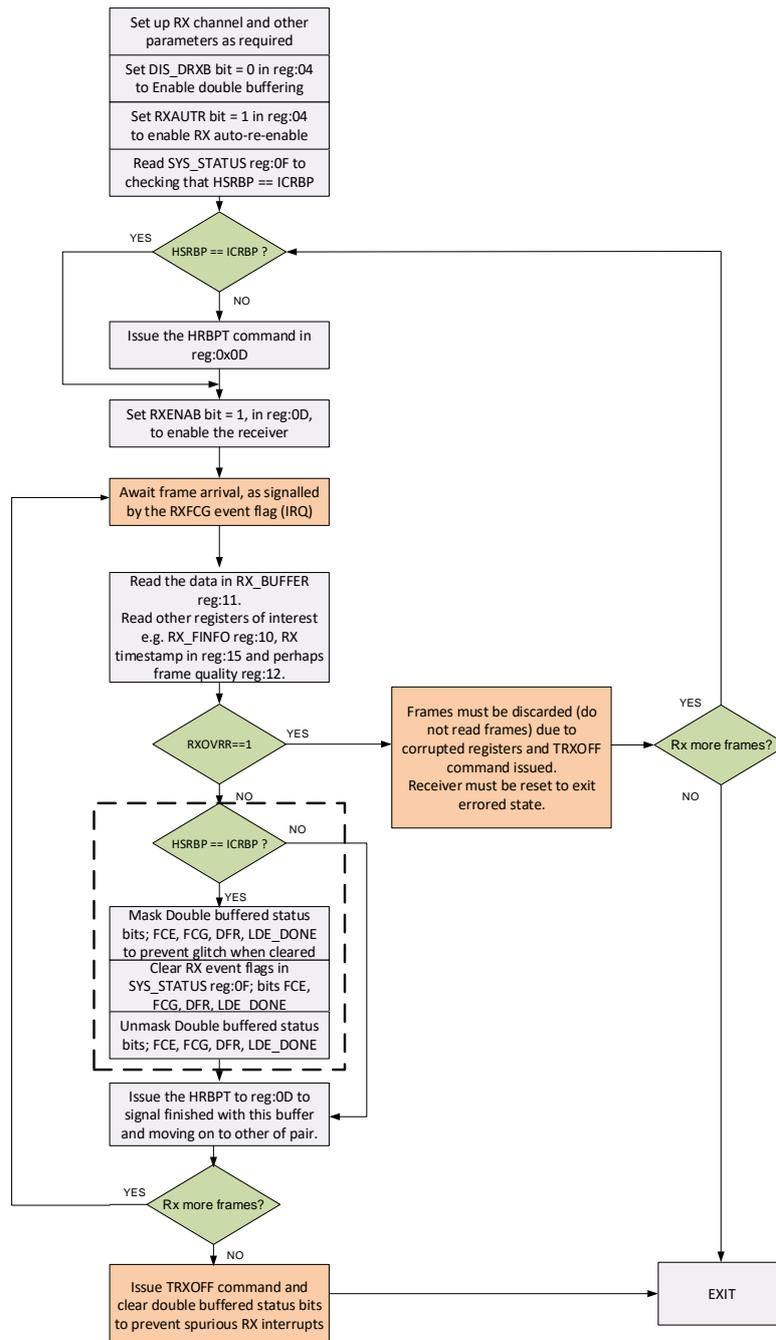
**Figure 14: Flow chart for using double RX buffering**
