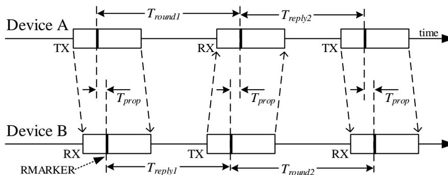
**Figure 38: Double-sided Two-way ranging with three messages**
