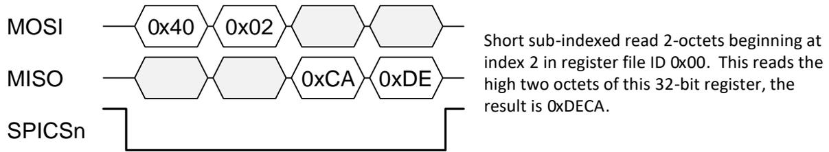
**Figure 5: Example short-indexed read of 3<sup>rd</sup> and 4<sup>th</sup> octets of register 0x00**
