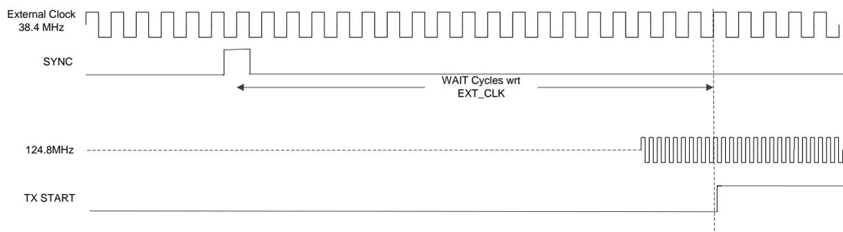
**Figure 24: Synchronised Transmission**
